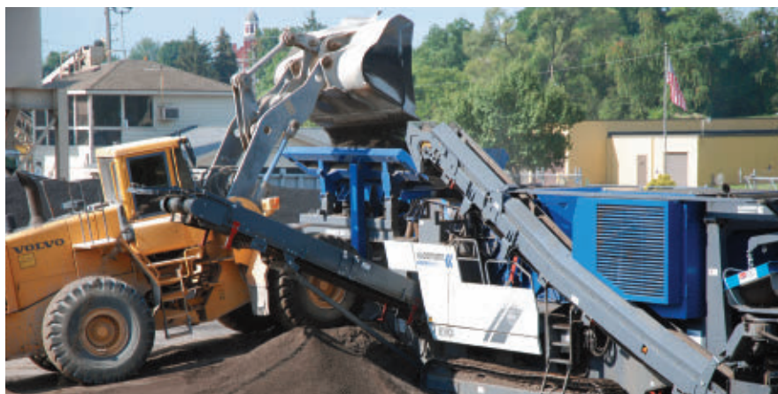
Beneficiation of raw milled RAP via crushing and screening boosts consistency and re-use of reclaimed material in mixes, via stockpiling of preferred aggregate sizes and average residual asphalt content after testing
