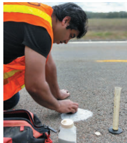
Hossam Abohamer field-tests chip seal sections constructed in District 58, Tensas Parish, La.
